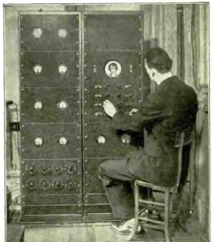
New style mixer and control panels, with image monitor, for television transmitting stations, designed by the Jenkins engineers.
