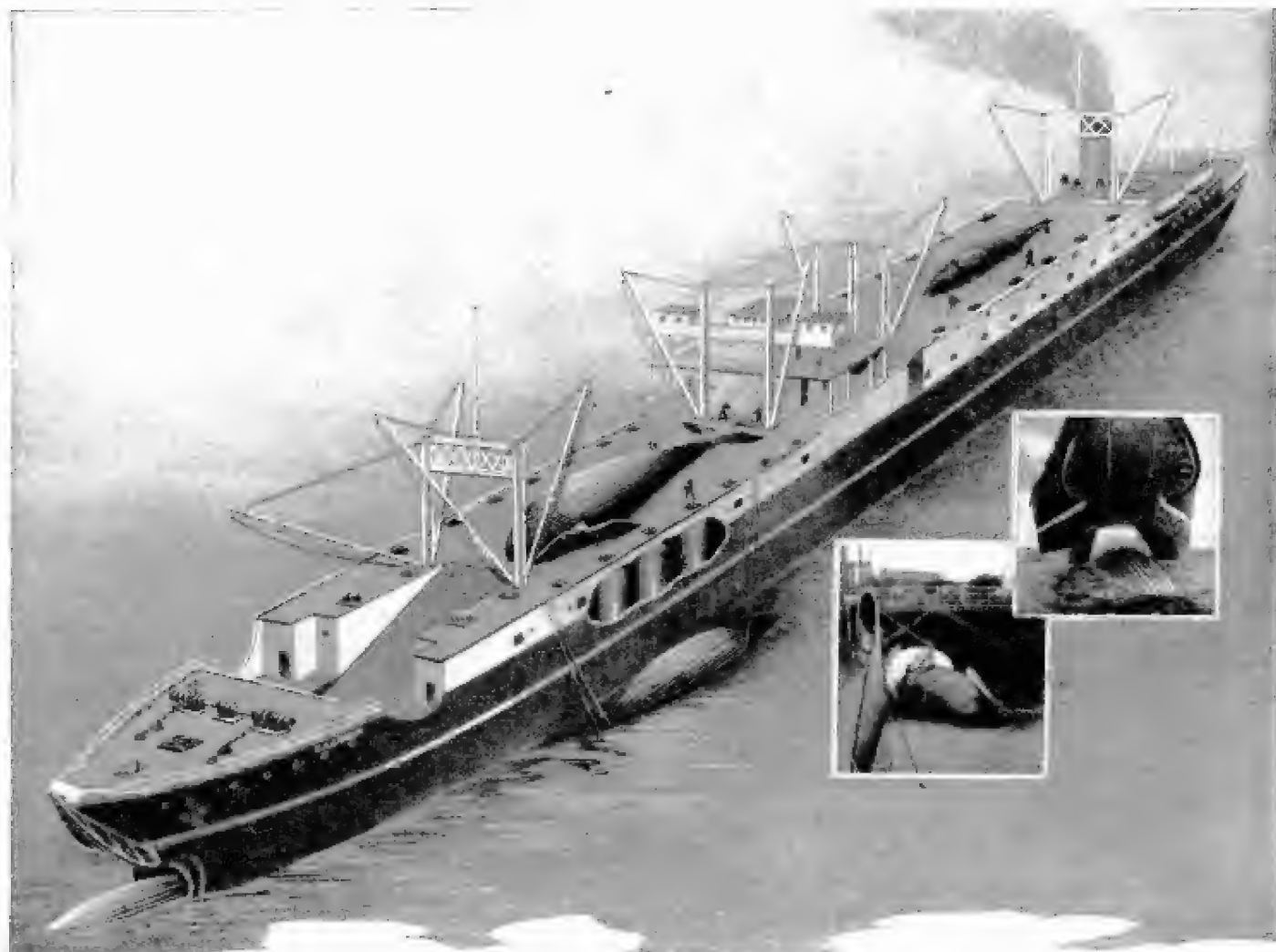
The whaling ship "C. A. Larsen" of Sandefjord, Norway, represents the very latest scientific development in a complete floating whaling depot and factory combined. This huge ship of some 17,000 tons dead weight "swallows" the dead bodies of whales which are brought in by the smaller "killer" boats.
