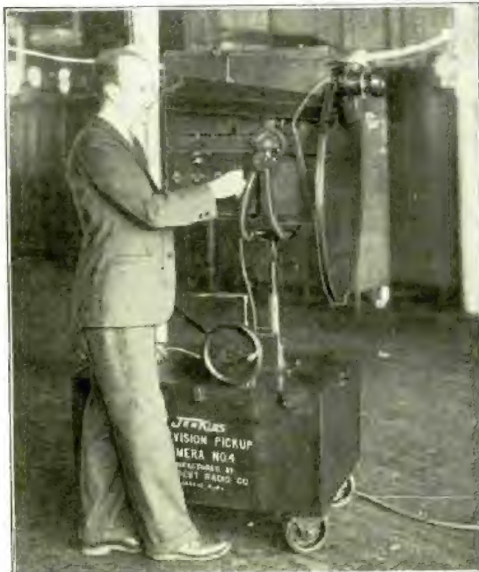
Latest model Jenkins "direct pickup" camera with mobile truck. The operator checks the image by looking into the scanner hood shown.
