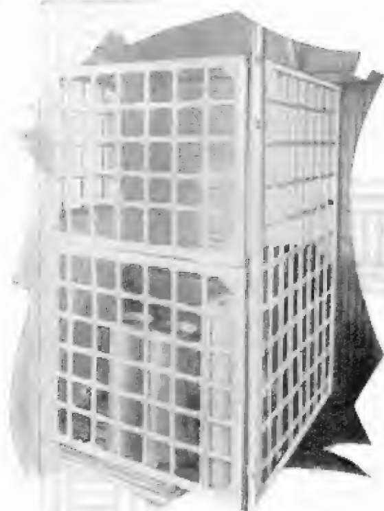
Food for the trip is stored in a metal bin which is shown above. The lattice work frame is entirely made of metal and riveted together.
