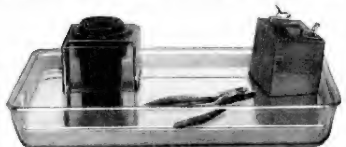
A glass ink well full of ink, a pair of cutting pliers and a "B" battery float in mercury. Observe how the "B" battery tips at an angle. Its construction makes it heavier on one side than on the other.
