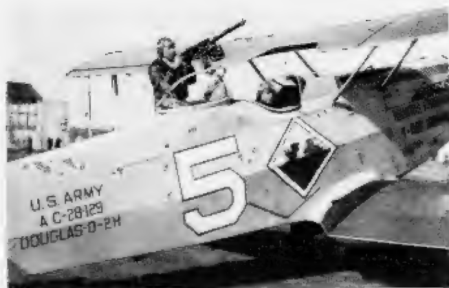
This aerial gun, a marvel of ballistical science, can pour forth 1200 bullets per minute at the maximum rate of fire.
