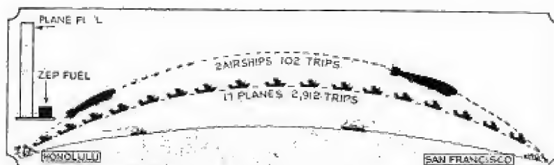
To transport 2,912,000 pounds per annum from Frisco to Honolulu, would require but 2 airships making 102 trips one way; 17 57-ton flying boats would be required to make 2,912 trips one way per annum.
