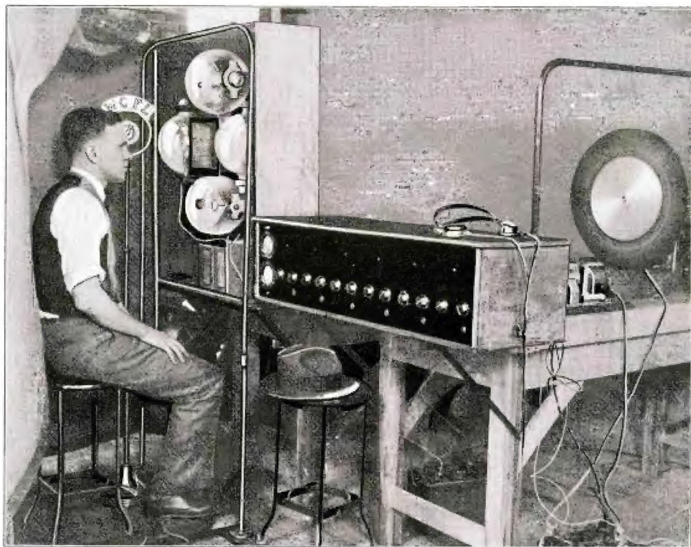
The photograph above shows the newest television transmitter recently demonstrated from broadcast station WCFL, Chicago. The apparatus was designed and constructed by two Chicago engineers, M. L. Hayes and U. A. Sanabria. The system is similar to the Bell Telephone Laboratory arrangement and large photo-
